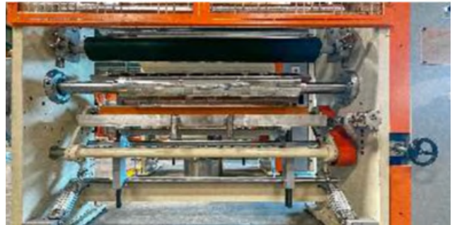
Shaftless Cylinder Chuckin / Driven Furnish Rollers / Impression Roller
