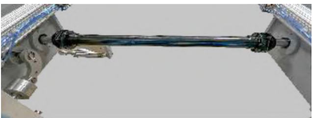
Line Shaft with Miki Pulley Couplings
