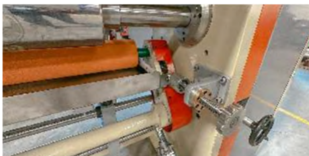
Micro adjustment setting system of Gap in Furnish Roller
