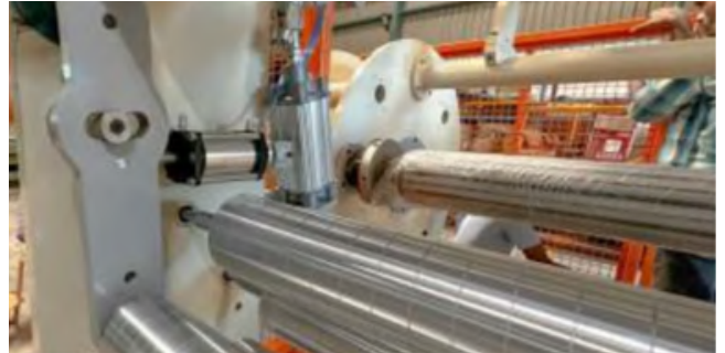
Frictionless Pneumatic Cylinders for Dancing Rollers
